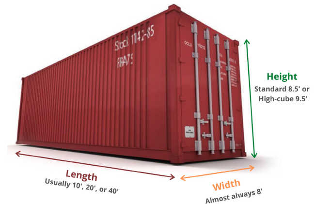
Figure 51: Shipping Container Dimensions
