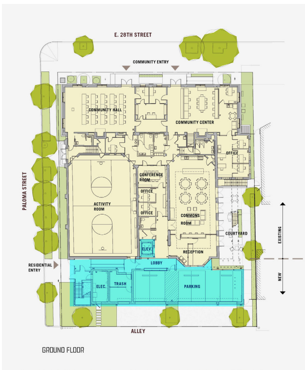
Figure 37: 28th St. Apartments. Ground Floor
