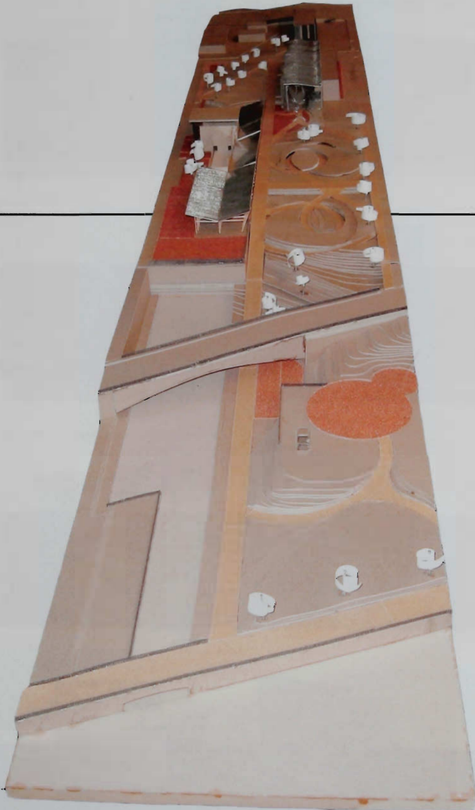
The site model here goes from Jefferson (top) down to the river (bottom). The model shows the topography change and the new channel being pulled in.
