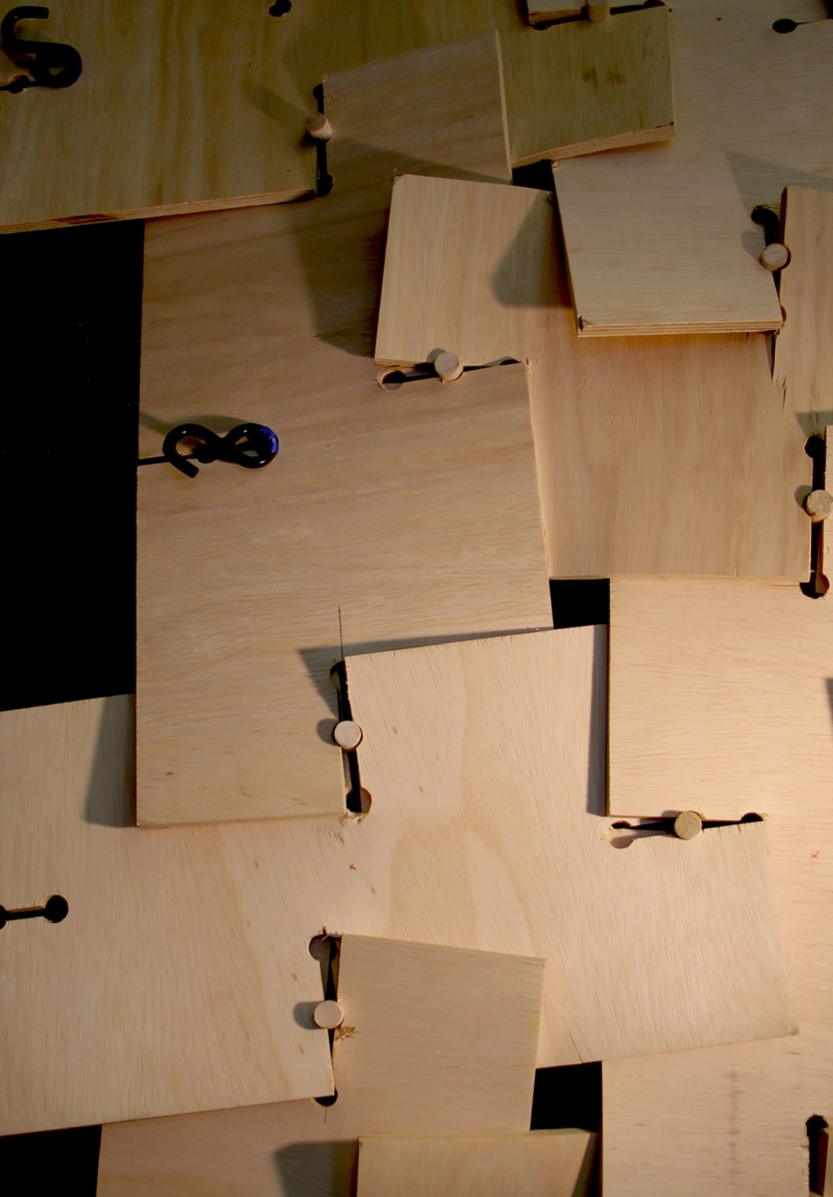
Pins appropriate, plywood too thick, aperture too small causing plywood to crush at bending moment
