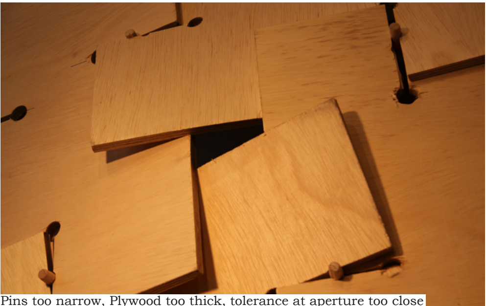
Pins too narrow, Plywood too thick, tolerance at aperture too close
