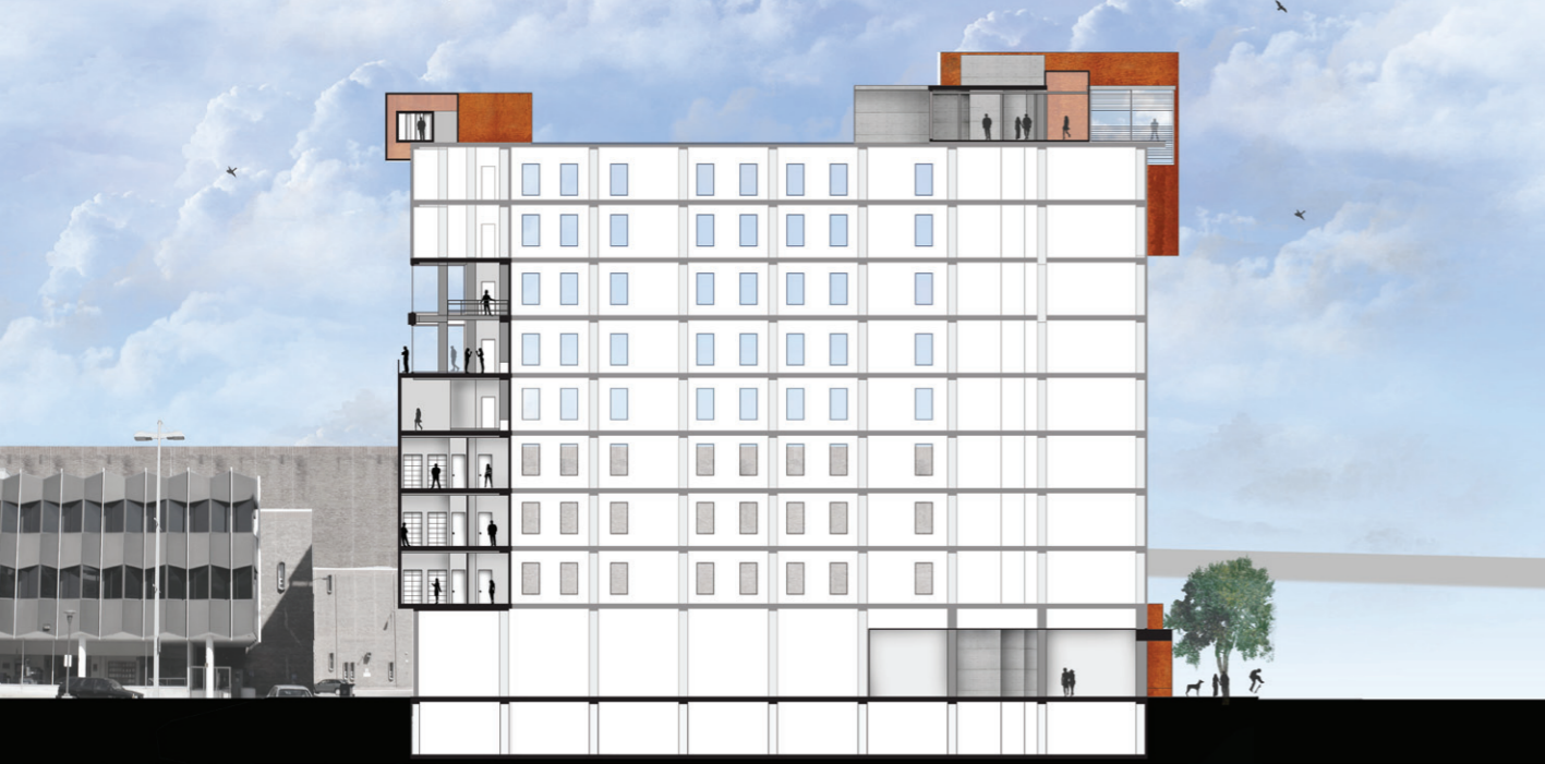
above: Section showing the organization of the dormitory space through the utilization of the building's existing structural bay
