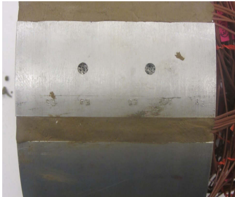
Figure 7. 8 Photograph of the Foam Sample Instrumented with Thermocouples
