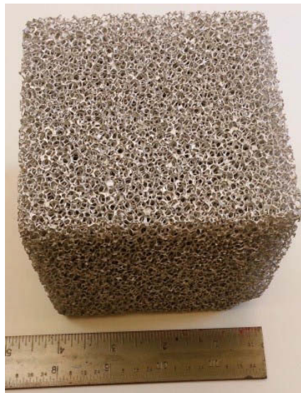
Figure 5. 3 10 PPI Duocel® Aluminum 6101 Alloy Metal Foam, 90.2 % Porous
