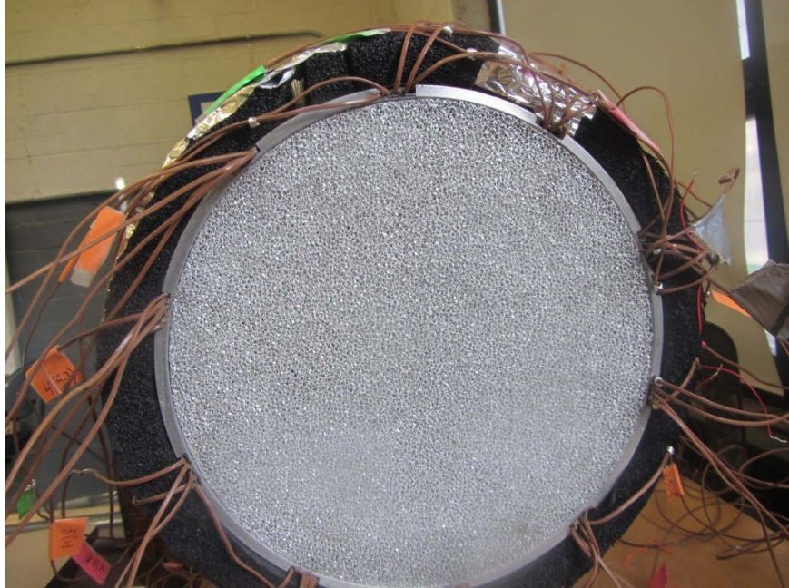
Figure 7. 12 Photograph of Sample Wrapped with the Insulation
