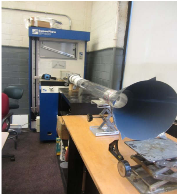
Figure 7. 11 Photograph of the Open-Loop Tunnel
