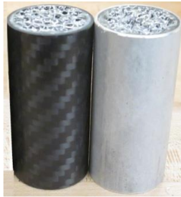
Figure 2 - Finished carbon fiber composite specimen on left and aluminum specimen on right.
