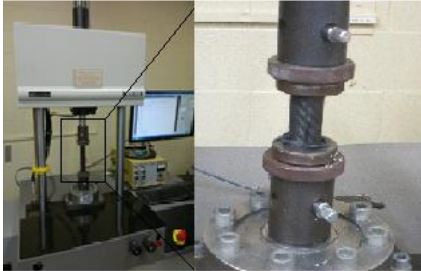
Figure 8 – Servo-hydraulic universal testing machine (left) and sample being crushed in uniaxial direction (right)
