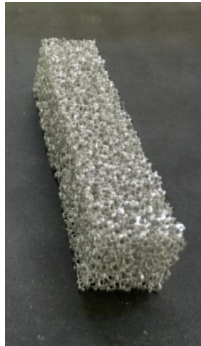
Figure 3 – Aluminum foam cut into 25X25X127 mm samples
